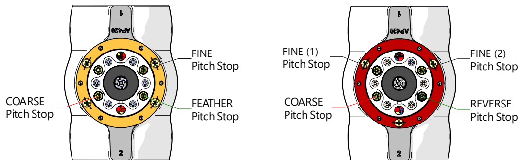
Figure 4. (Left) Layout of adjustable pitch stops in a 2-port feathering hub (AH-420CF shown).
